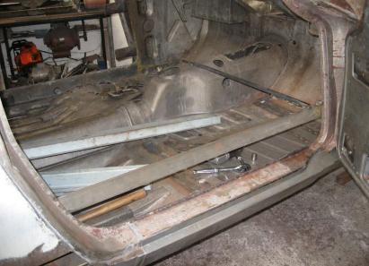
minor corrosion in the corners of the front footwells. By replacing the front outer floor sections, it meant that replacement of the outriggers below the floor was
