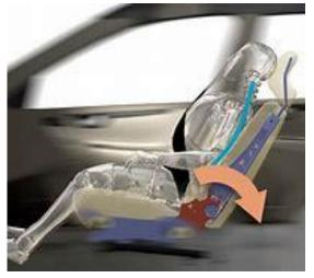
piece of metal inside the backrest hinge deforms, absorbing more energy. The hinge piece needs to be replaced after having been deployed/
